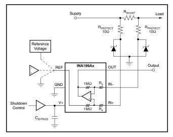
Figure 24. INA199Ax Transient Protection Using Dual Zener Diodes
