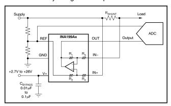
Figure 23. Sensing INA199Ax to Cancel Effects of Impedance on the REF Input
