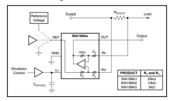
NOTE:  $1M\Omega$  paths from shunt inputs to reference and INA199Ax outputs.
