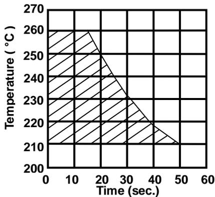
(4) Standard Temperature Profile for Soldering
