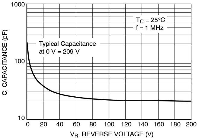
Figure 5. Typical Capacitance
