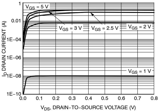
**Figure 8. Output Characteristics**
