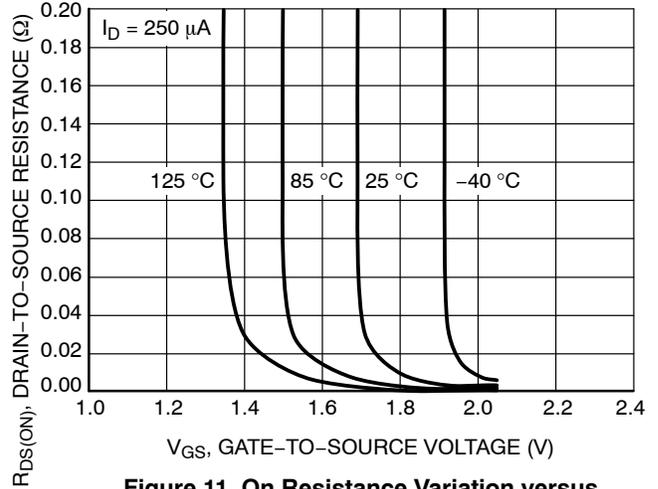
**Figure 11. On Resistance Variation versus Gate-to-Source Voltage**
