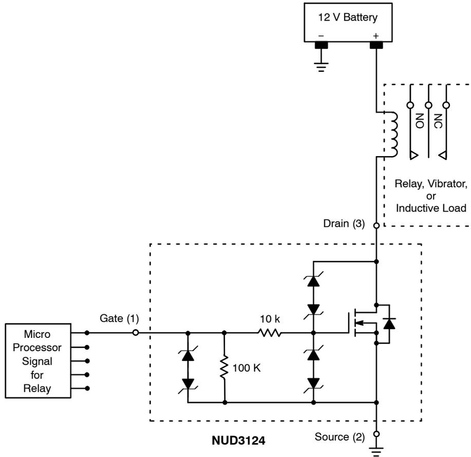
Figure 14. Applications Diagram
