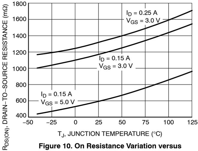
**Figure 10. On Resistance Variation versus Junction Temperature**
