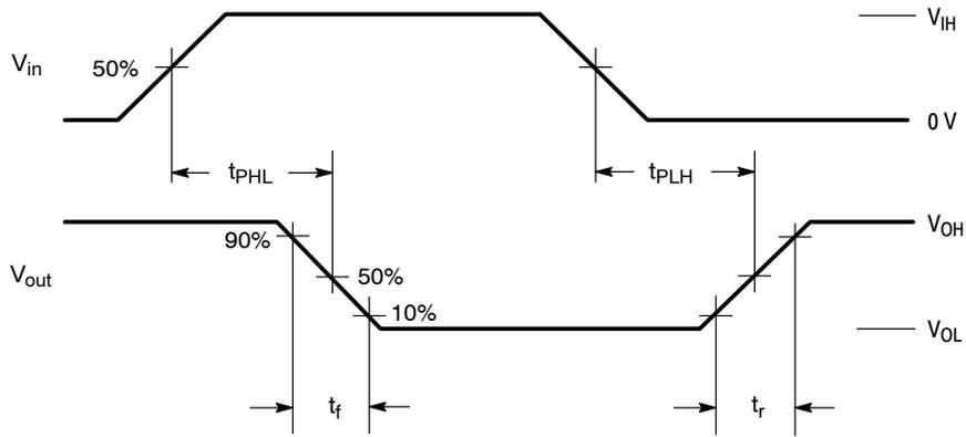
Figure 1. Switching Waveforms
