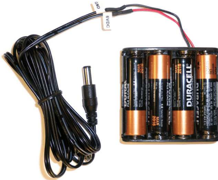
Figure 70. Recommended Power Supply for ADS1299EEG-FE
