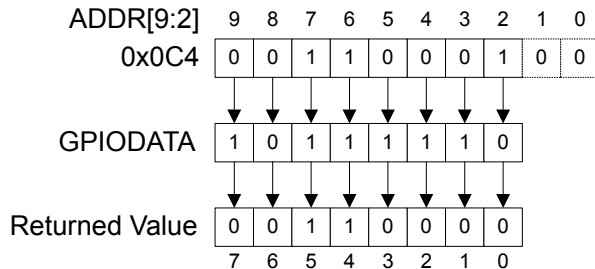
Figure 9-3. GPIODATA Read Example
