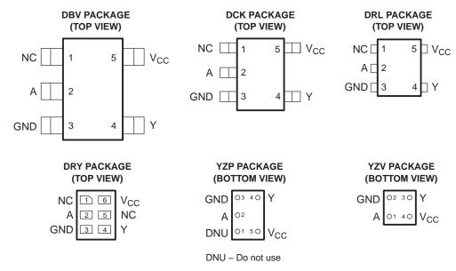
NC – No internal connection See mechanical drawings for dimensions.
