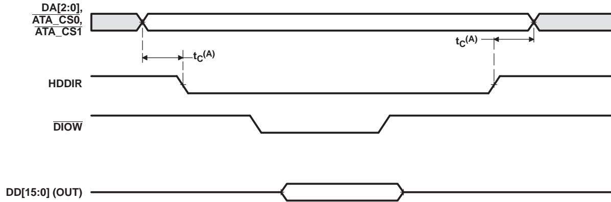
Figure 6-38. ATA/CF HDDIR Taskfile Write/Single PIO Write Timing
