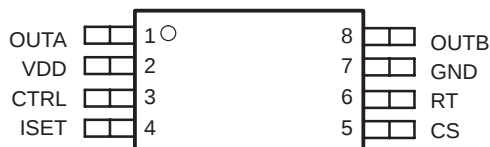
PW PACKAGE (TOP VIEW)
