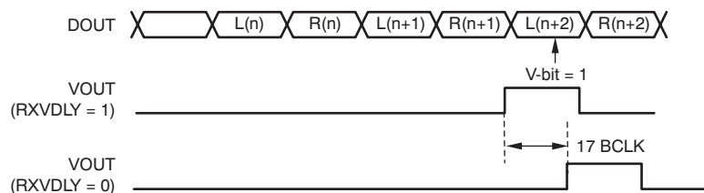
Figure 25. RXVDLY and VOUT Timing
