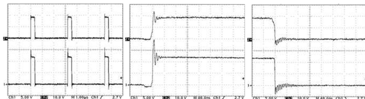
Figure 20. HDRV and SW Node of 1.2-V Output at 12 Vin, 20-A Output
